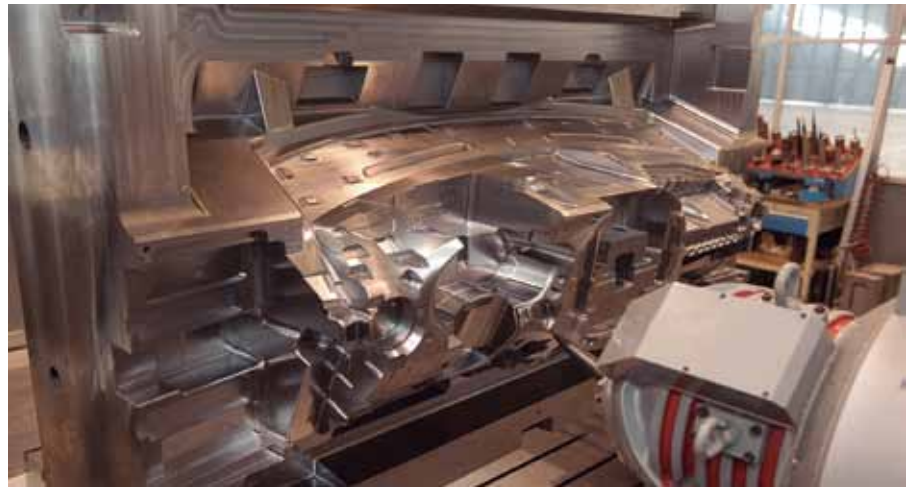
Finish milling of the core of a injection mould, ready to produce car dashboards. Photo by Geco Moldes
